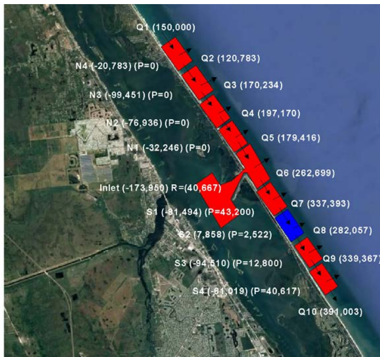
Figure 28. Annualized sediment budget for the summer 2010 to summer 2013 time period. Values on the west of the barrier island indicate sand volume changes and values on the east indicates calculated sand flux rate in cubic yards per year. P= annualized placement quantities and R = annualized value of sand removed from the sand trap. Blue cells indicate sand volume increase whereas red cells indicate sand volume loss. Offshore transport from each of the cells was required to balance the sand budget.
