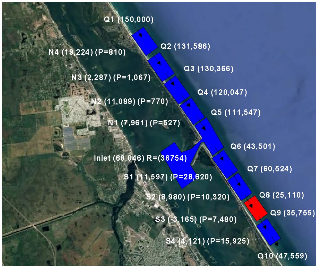
Figure 25. Annualized sediment budget for the summer 2007 to summer 2017 time period. Values on the west of the barrier island indicate sand volume changes and values on the east indicates calculated sand flux rate in cubic yards per year. P= annualized placement quantities and R = annualized value of sand removed from the sand trap. Blue cells indicate sand volume increase whereas red cells indicate sand volume loss.
